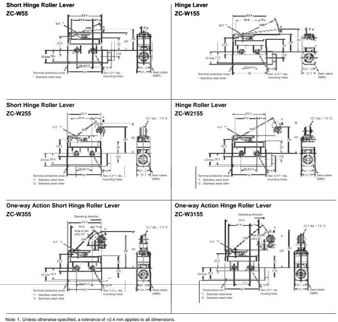
Note: 1. Unless otherwise specified, a tolerance of ±0.4 mm applies to all dimensions.
